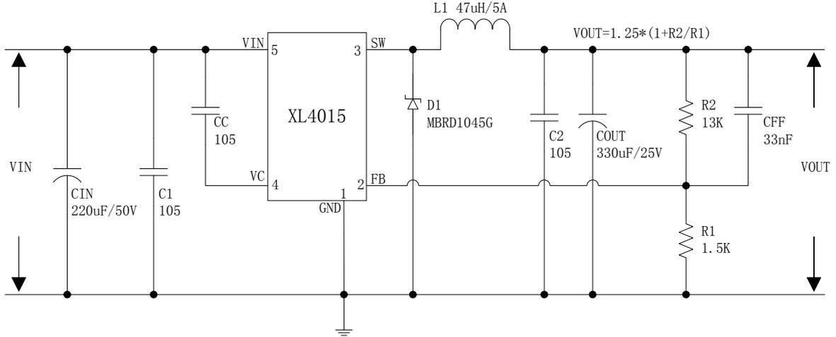
Figure7. XL4015 System Parameters Test Circuit (VIN=15V~36V, VOUT=12V/4A)
