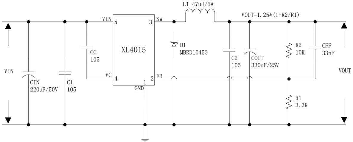
Figure5. XL4015 System Parameters Test Circuit (VIN=8V~36V, VOUT=5V/5A)
